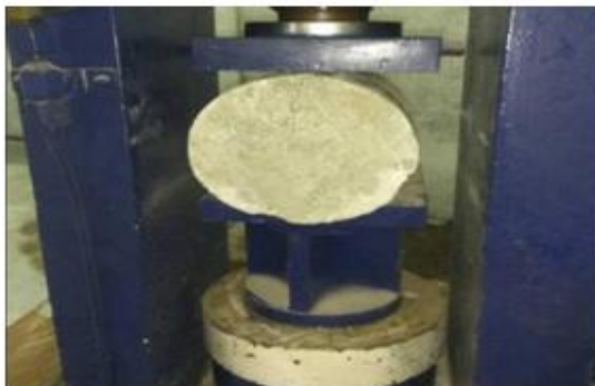
Figure.8. split tensile test for fibers
