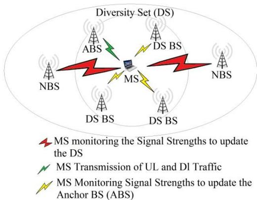
**Figure.2. Fast Base Station Switching**
