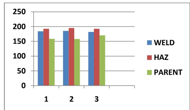
Figure.9. Vickers Hardness test
