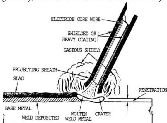
**Figure.1. Shielded Metal Arc Welding**
