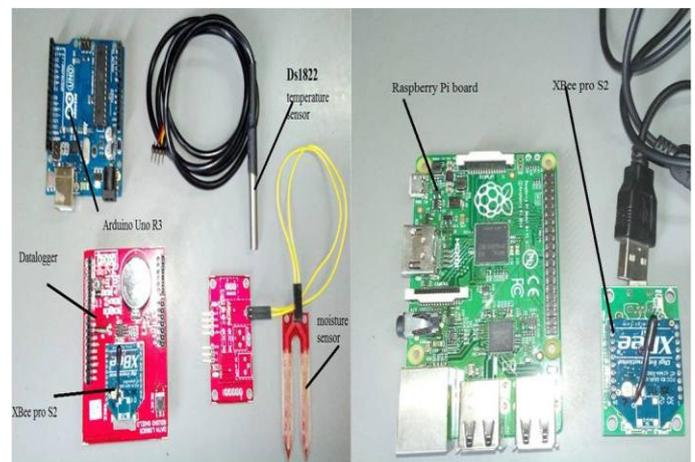
Figure.6. WSN and coordinator node components
