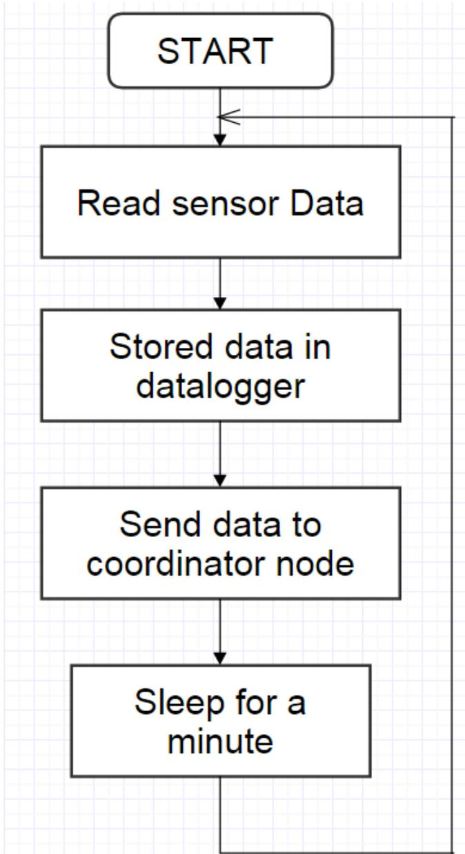
Figure.4. Sensor node flowchart for end device
