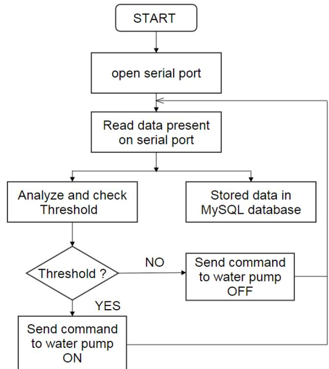
Figure.5. Coordinator node flowchart for end device
