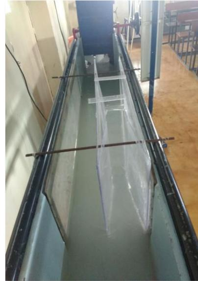
**Figure.7. Miniature Venturiflume In Floating Condition (50%)**
