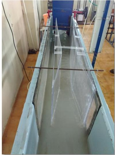
**Figure.6. Miniature Venturiflume In Floating Condition (75%)**
