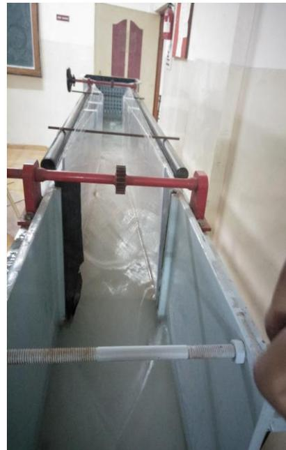
Figure.5. Conventional Venturiflume In Floating Condition
