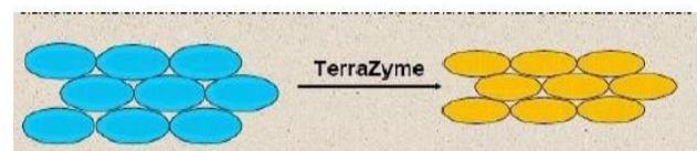
Bio-Enzyme(Terrazyme) replaces adsorbed water with organic cat-ions, thus neutralizing the negative charge on a clay particle.
