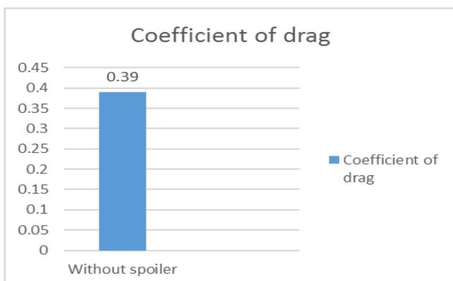
The graph shows the maximum value of coefficient of drag is 0.39 when vehicle is without spoiler
