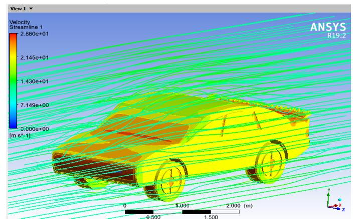
Figure. 5.4 Velocity flow regime at 40km/h (with spoiler)
