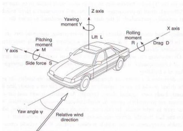
**Figure.1.3 Aerodynamic Forces and Moments Acting On a Vehicle**
