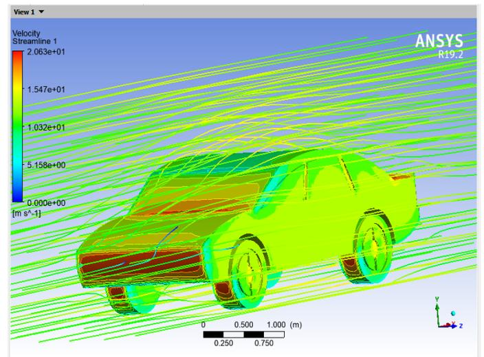
Figure.5.3 Velocity Flow Regime at 40km/h (without spoiler)
