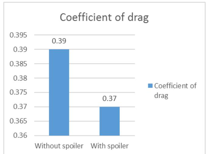
The graph shows the variation of coefficient of drag when vehicle is without spoiler and with spoiler
