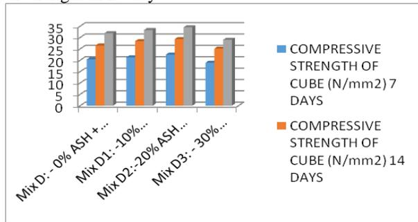
Figure.4. Compressive strength of Cube
