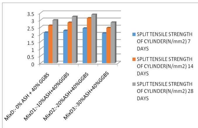
Figure. 5. Split Tensile Strength of Cylinder
