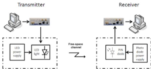
Figure.1. shows VLC Transmitter and VLC Receiver.
