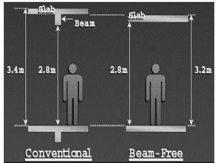
Figure.2. Comparison of Flat and Conventional Slab
