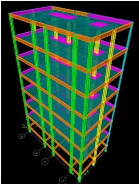
Figure.4. 3D View of Flat slab building
