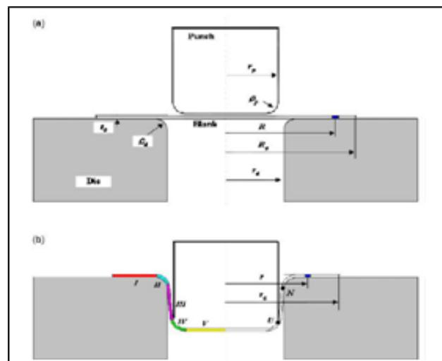
**Figure.1. Deep drawing for a circular cup (a) initial stage and (b) Intermediate stage.**
