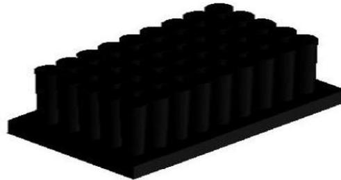
Figure.4. (c) Isometric view of Modified pin fin heat sink (two degree expansion)
