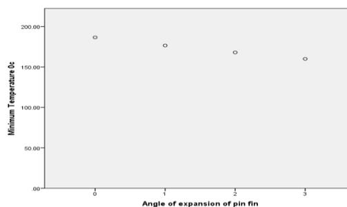
Graph.1.(a) minimum temperature and angle of expansion of pin fin
