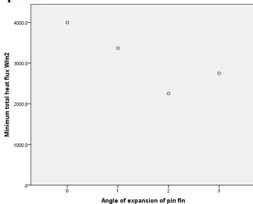
**Graph.1.(c) minimum total heat flux and angle of expansion of pin fin**
