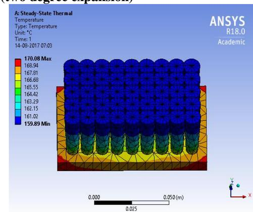
Figure.5.(d) Temperature of Modified pin fin heat sink (three degree expansion)
