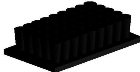
Figure.4.(d) Isometric view of Modified pin fin heat sink (three degree expansion)
