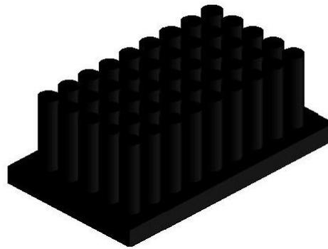
Figure.4.(a) Isometric view of Conventional pin fin heat sink (zero degree expansion)
