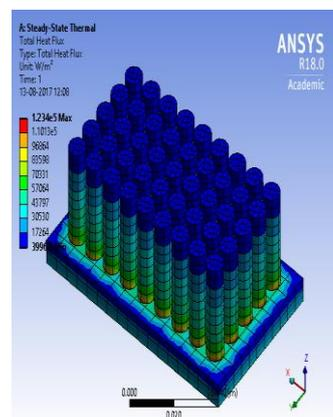
Figure.6.(a) Total heat flux of Conventional pin fin heat sink (zero degree expansion)
