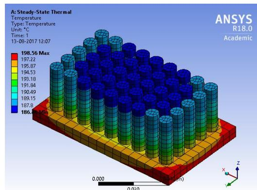
Figure.5.(a) Temperature of Conventional pin fin heat sink (zero degree expansion)
