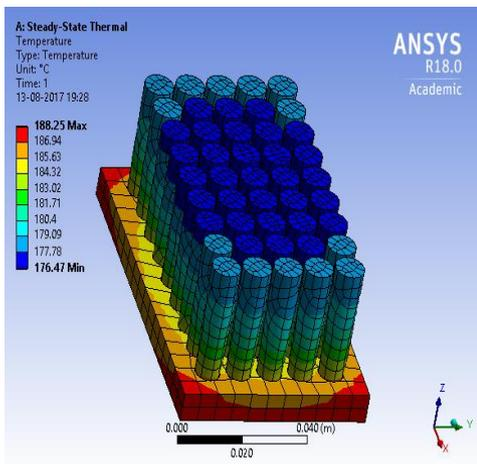
Figure.5.(b) Temperature of Modified pin fin heat sink (one degree expansion)
