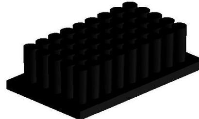
Figure.4.(b) Isometric view of Modified pin fin heat sink (one degree expansion)
