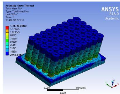
Figure.6.(c) Total heat flux of Modified pin fin heat sink (two degree expansion)
