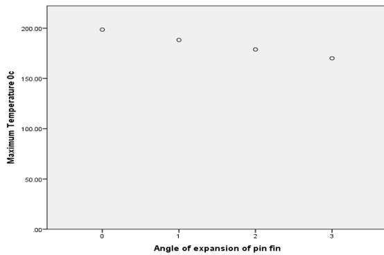
**Graph.1.(b) maximum temperature and angle of expansion of pin fin**
