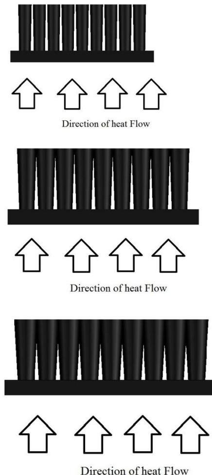
Figure. 2. The modified pin fin heat sink with 1 degree 2 degree and 3 degree of expansion (Front view)
