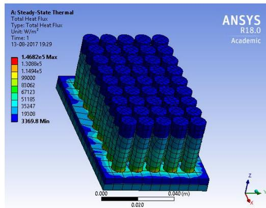
Figure.6.(b) Total heat flux of Modified pin fin heat sink (one degree expansion)
