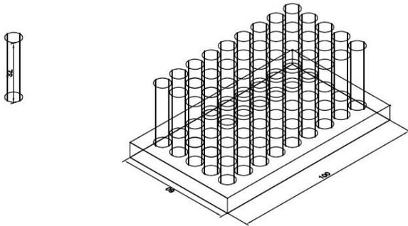
Figure.3. Geometric parameters of heat sink (isometric view)
