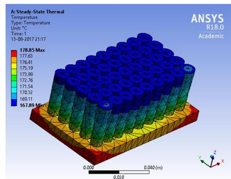
Figure.5. (c) Temperature of Modified pin fin heat sink (two degree expansion)
