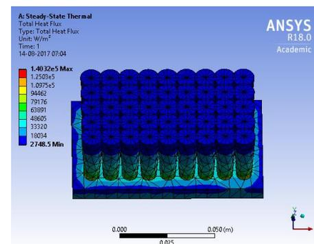
Figure.6.(d) Total heat flux of Modified pin fin heat sink (three degree expansion)
