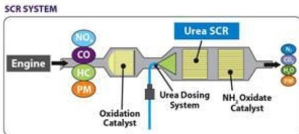
The catalytic converter is a device placed in the exhaust pipe, which converts hydrocarbons, carbon monoxide, and NO<sub>x</sub> into less harmful gases by using a combination of platinum, palladium and rhodium as catalysts.
