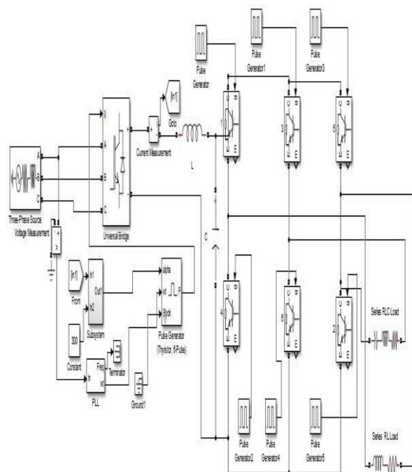
Figure.4. Converter-Inverter Bridge configuration.
