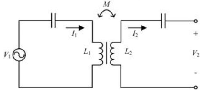
Figure.4. Basic circuit model of wireless power transfer system.
