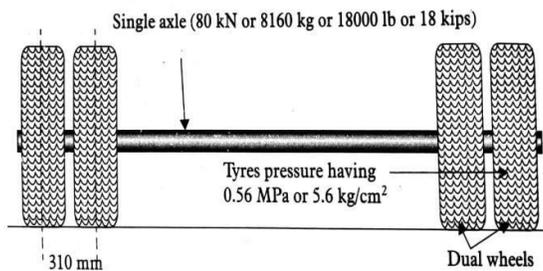
The above picture shows the details of the Indian standard axle. With the standard axle of 80 kN resting on dual tyres on axle configuration, it can be assumed that the axle on single tyres is 6.5 kN. In line with above assumptions to the data of table no 3, the respective overloaded axles are computed as:
