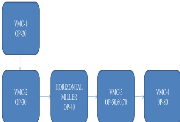
Fig Recommended arrangement of machines
