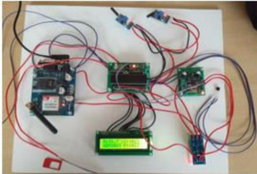
The system is used to monitor the windmill through wireless communication system through an Internet of things. This system monitors the Temperature, vibration of the windmill. This system is mainly used to detect the cable twist occur in the windmill by using the flex sensor. The application used in the mobile phone for the monitoring the values obtained by the sensor is monitored by an UBIDOTS.
