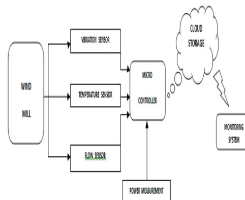
The system starts working when the PIC microcontroller gets the input from all the three sensors. The temperature and the vibration of the machine is calculated and displayed on the smart phone using the database from the IoT. This data can be stored in the cloud and can be used for future reference.
