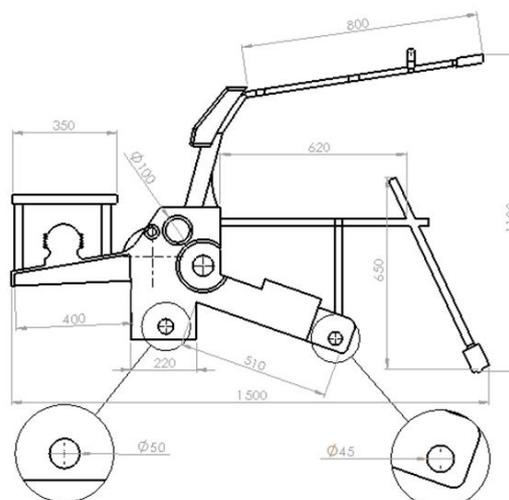
Figure.2.2 Main Frame (Side View)
