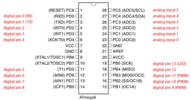
The Atmel®AVR® core combines a rich instruction set with 32 general purpose working registers. All the 32 registers are directly connected to the Arithmetic Logic Unit (ALU), allowing two independent registers to be accessed in one single instruction executed in one clock cycle. The resulting architecture is more code efficient while achieving throughputs up to ten times faster than conventional CISC microcontrollers.
