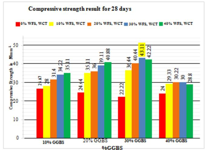
**Fig: 4.1. Effect of GGBS and WFS, WCT percentages on 28<sup>th</sup> days compressive strength**
