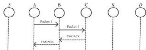
Fig. 1. Each node is required to send back an acknowledgment packet to the node that is two hops away from it.
