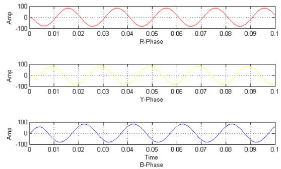
**Figure.1.shows the filtered output waveform of the NPC inverter.**
