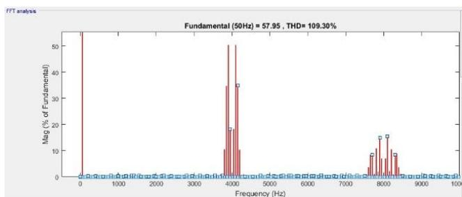
Figure.6.5. THD in Line Voltage of 3-phase 2-level inverter.
