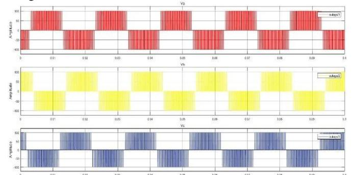
**Figure.6.3. Output Waveform of the two level three phase inverter without filter.**
