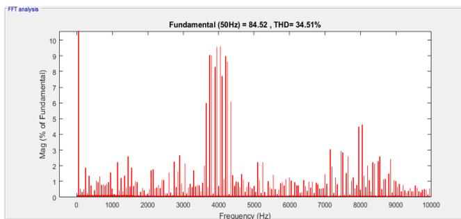
Figure.6.4. THD in Line Voltage of 3-phase 3-level inverter.
