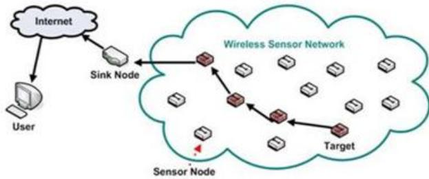
Figure.1. Wireless sensor network
