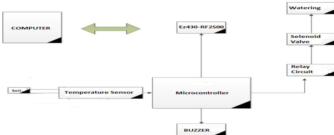
Figure. 2. Greenhouse Watering System with Microcontroller
