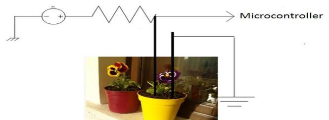
**Figure.1. Soil Moisture Probe [5]**
