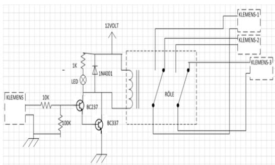
Figure. 3. Relay Circuit [5]
