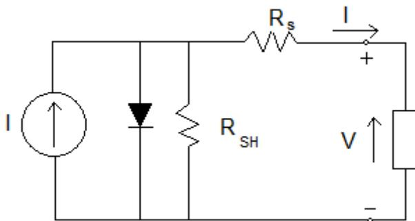
Figure.2. Single diode model of a PV cell
