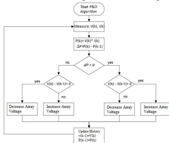
Figure. 3. Flowchart of Perturb & Observe algorithm
