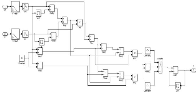
**Figure. 10. Sub-block model for the Model Predictive MPPT controllers**
