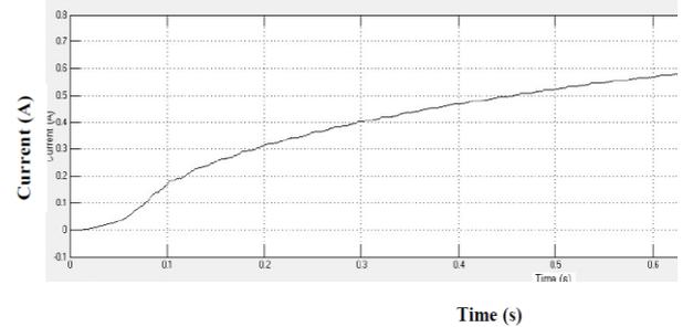
**Figure. 13. OUTPUT Current waveform for P & O MPPT controllers**
