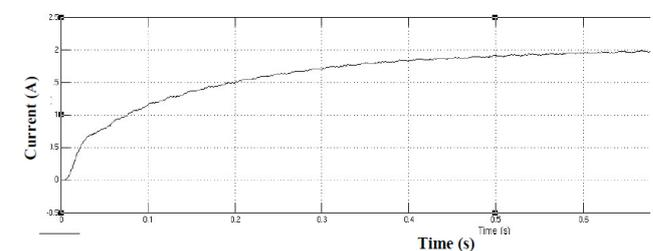
**Figure.16. OUTPUT Current waveform for MPC MPPT controllers**
