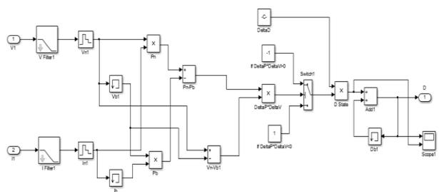
Figure.4. Sub-block model for the conventional P & O MPPT controllers
