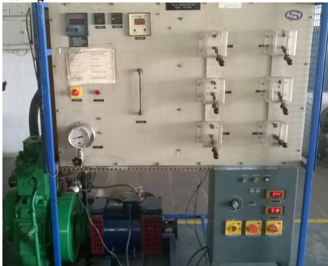
Figure.2.4 stroke single cylinder diesel engine set up with generator loading
