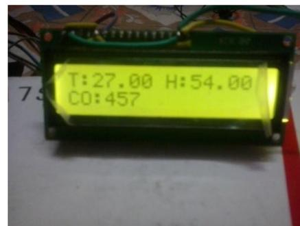
Fig. 9.1 Output displayed on LCD display
