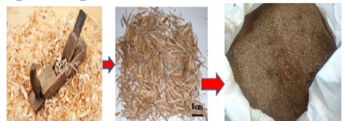
Figure.2. Sawdust in its raw state converted to Sawdust Ash
