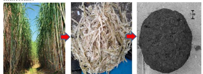
Figure.1. Sugarcane converted and processed into Sugarcane bagasse ash
