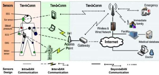
Figure.1. A three-tier architecture for WBANs
