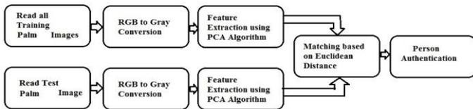
Fig.1. Palm vein authentication using Principal Component Analysis
