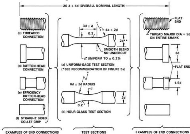
Figure.1. Standard Dimension of ASTM E – 606
