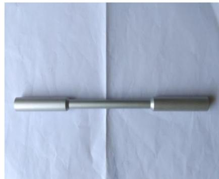
Figure.4. Specimen of Coated (Anodizing With Sand Blasting)
