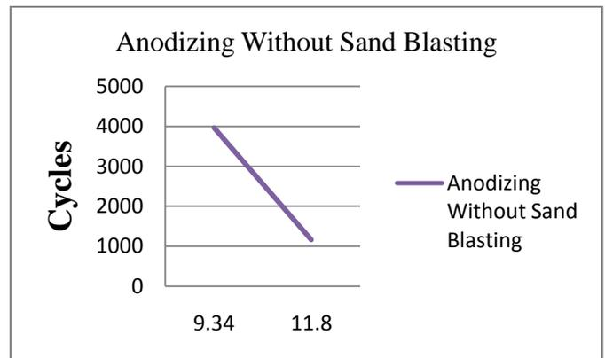
**Figure.12. Anodizing without Sand Blasting (Cycle vs Load)**
