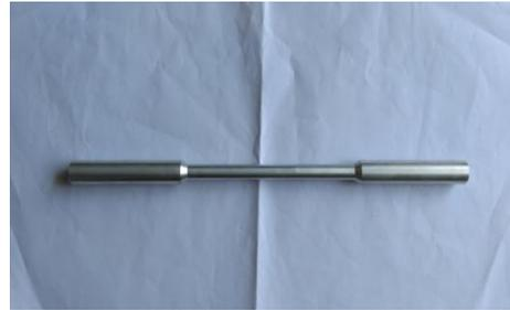
Specimen of Uncoated Material
