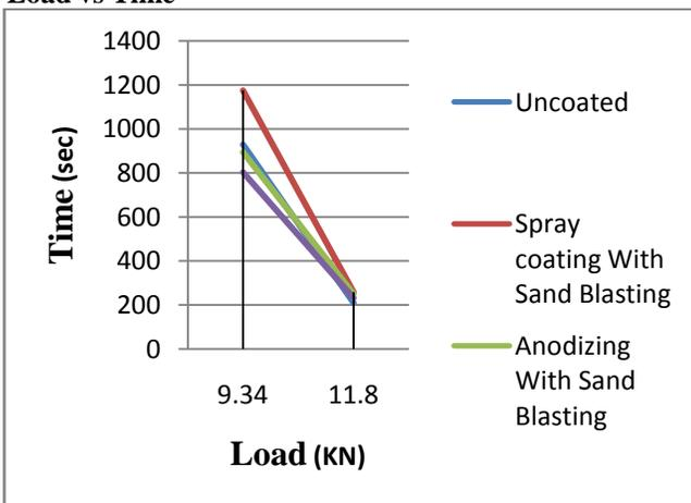
The graph is plotted based on the time and load. This graph is represent on uncoated, spray coating with sand blasting, anodizing with sand blasting, anodizing without sand blasting, aluminium alloy 6063 specimen. The load is taken as 9.34 and 11.8 KN. The value should be taken as per the mean value of two set of trials. Increase in load may decreases the time
