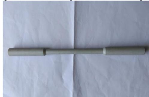
Figure.5. Specimen of Coated (Anodizing Without Sand Blasting)
