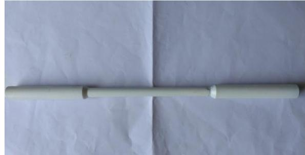
Figure.3. Specimen of coated (Spray Coating With Sand Blasting)
