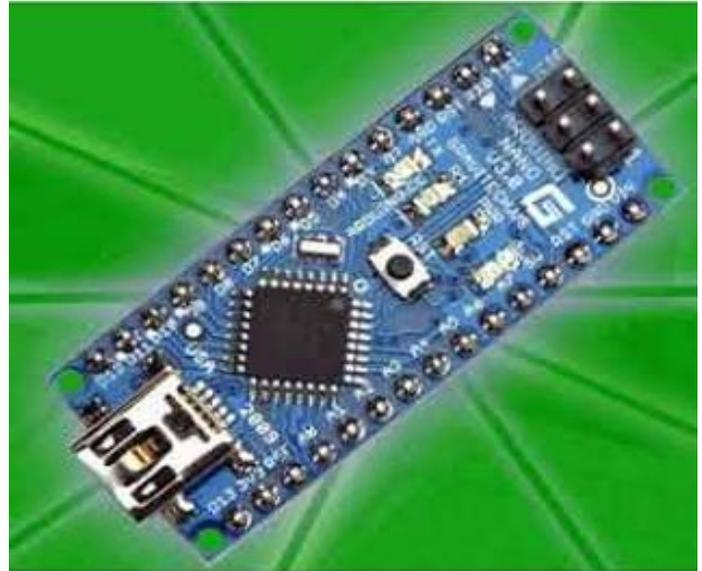
**Figure.2. Arduinonano3.0 microcontroller**
