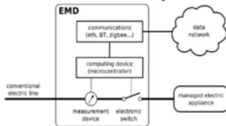
**Figure.2. Block diagram of the general EMD structure.**
