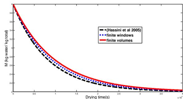
**Figure.6.**Comparison Of the Experimental Curve, the Curve of Simulation by the Method of Finite Volumes and Finite Windows
