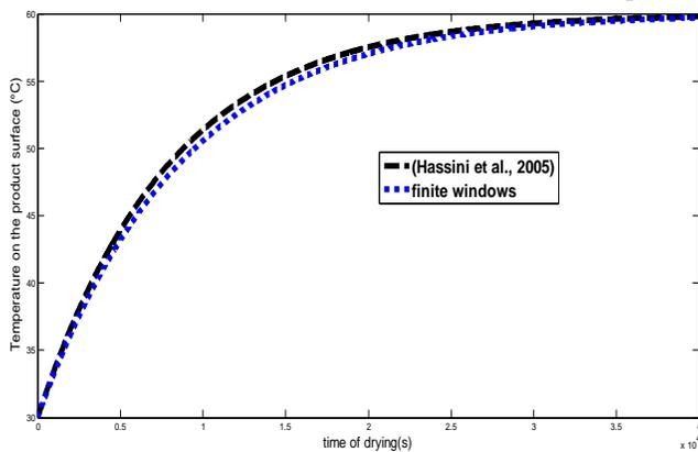
**Figure.2.** Comparison of the experimental values of hassini *et al.*, (2005) and of the values simulated by the finite windows method
