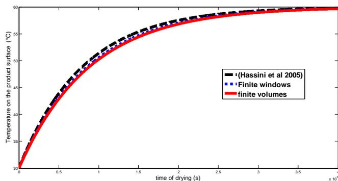
**Figure.3.** Comparison of the experimental curve of hassini *et al.*, (2005) and of the curve simulated by the method of finite volumes and finite windows method
