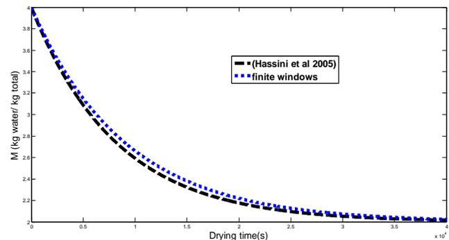
**Figure.5.**Comparison Of the Experimental Curve and the Curve of Simulation
