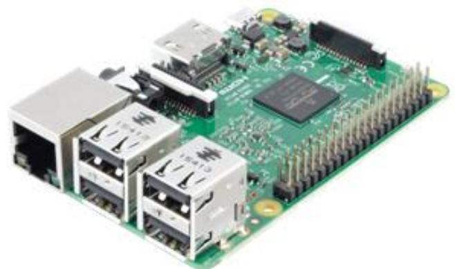
Raspberry Pi controller is used here. As the Raspberry Pi 3 supports HD video, you can even create a media center with it. It is fully HAT compatible and has 1GB RAM so you can run bigger and more powerful applications. Micro SD slot for storing information and loading operating systems. Broadcom BCM2387 ARM Cortex-A53 Quad Core Processor powered Single Board Computer running at 1.2GHz. It has 40 pins extended GPIO to enhance projects.
