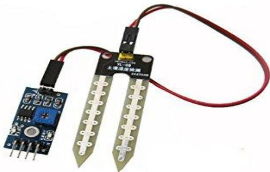
Soil moisture sensors typically refer to sensors that estimate volumetric water content. It used copper electrodes to sense the moisture content of the soil. Its range is 0 to 45% volumetric water content in soil. It operates between  $-40^{\circ}\text{C}$  to  $+60^{\circ}\text{C}$ .
