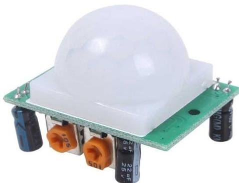
A Passive Infrared sensor is an electronic sensor that measures Infrared radiation being emitted from objects in its field of view. A PIR based motion detector is used to detect the motion of people, animals, or other objects. They are commonly also called as Passive Infrared Detector
