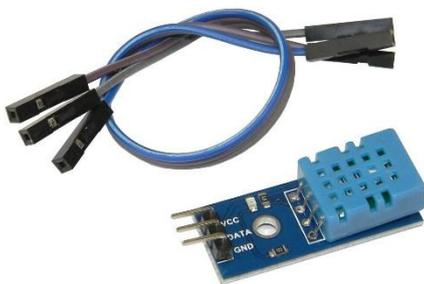
The DHT11 is a low-cost temperature and humidity sensor. It therefore measures both moisture and air temperature. It isn't the fastest sensor around but its cheap price makes it useful for experimenting or projects where you don't require new readings multiple times a second. The device only requires three connections to the Pi.
