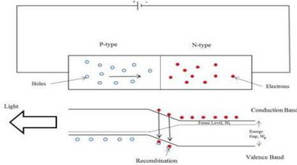
**Figure 2.2 LED PN- junction biasing arrangement**
