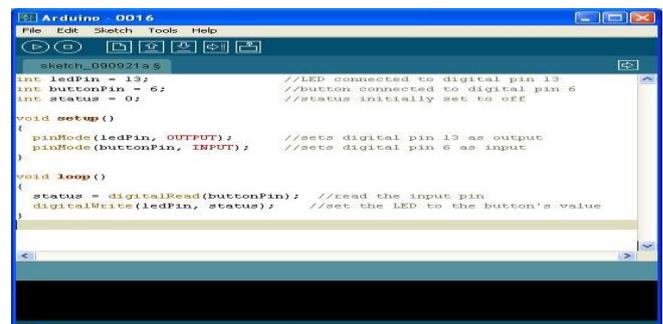
**Figure 5.7 Arduino Code using push button is used to turn on the LED**
