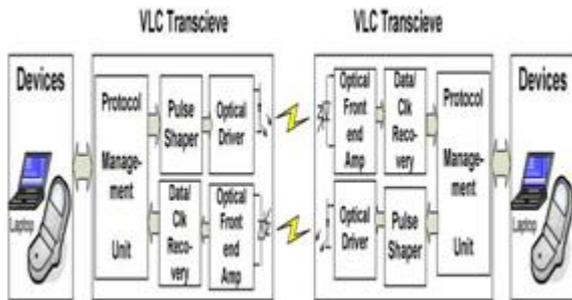
Figure 4.2: General architecture for a full duplex VLC system
