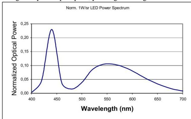
**Figure 2.3: Normalized optical spectrum of a white LED**
