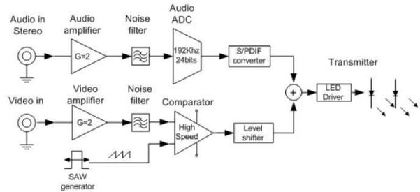
Figure 4.3 Architecture of the dual-use optical communication
