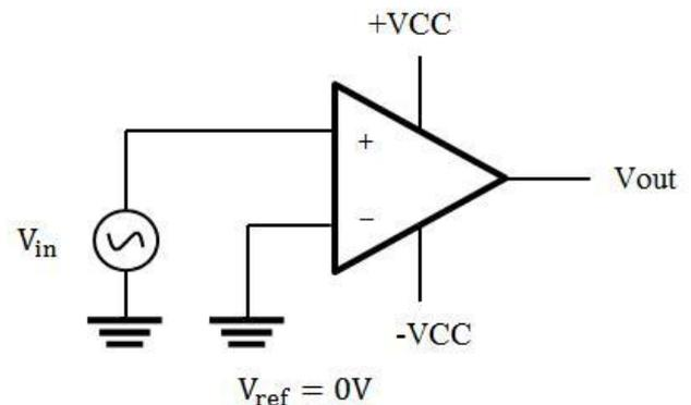
**Figure 3.1: Voltage Comparator configuration**
