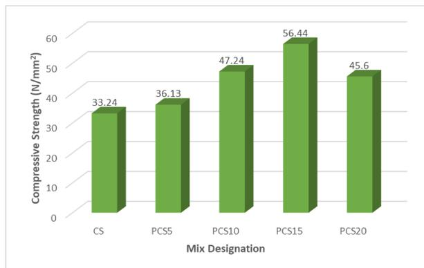
**Figure.3. Comparison of Compressive Strengths**
