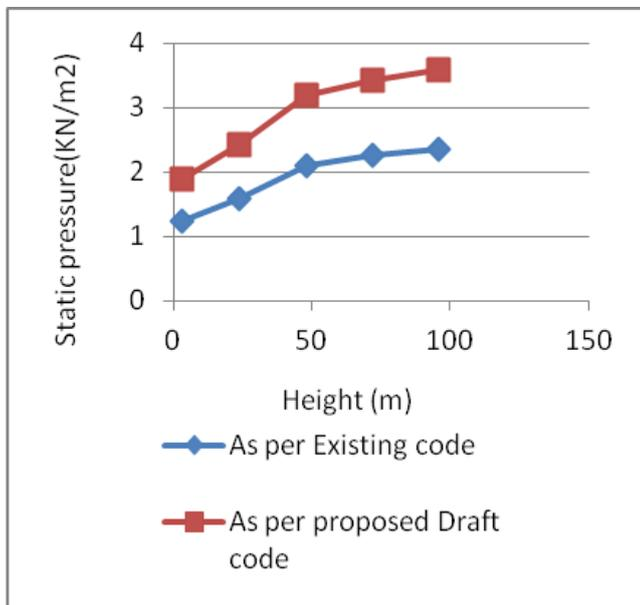
Figure.3. Variation of Static Wind Pressures with height located at Visakhapatnam
