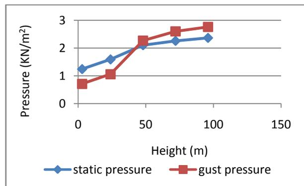
**Figure.6. Variation of Static pressure and Gust Pressures with height as per Existing IS code [2]**
