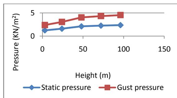
**Figure.7. Variation of Static pressure and Gust Pressures with height as per proposed draft code [4]**
