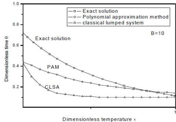
**Figure.3. Comparison of solutions of PAM, CLSA and Exact solution for a slab having internal heat generation**
