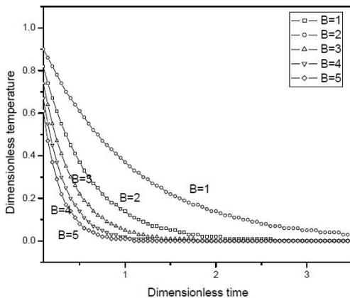
**Figure.2. Variation of average temperature with dimensionless time, for B=1 to 5 for a slab**
