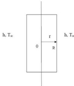
Figure.2. Schematic of slab
