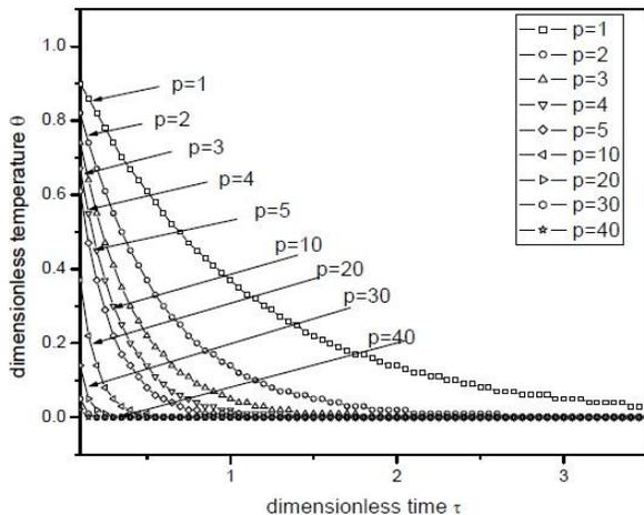
**Figure.1. Variation of average temperature with dimensionless time, for P=1 to 40 for a slab.**
