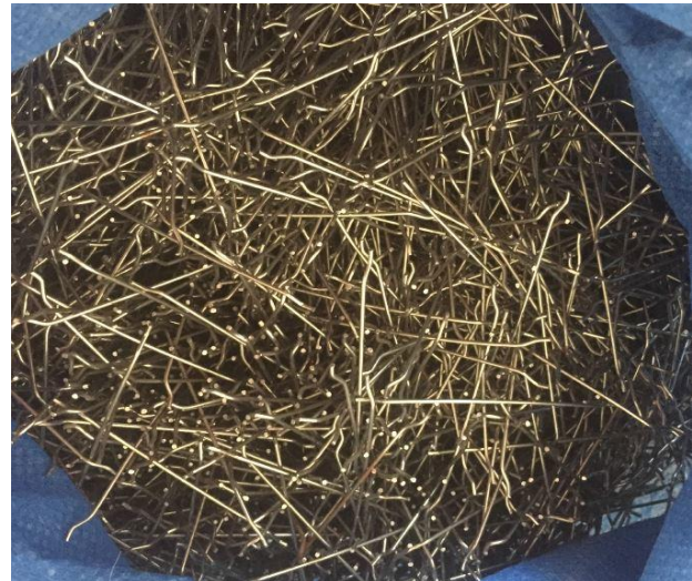
Figure.2 Steel Fibres with Aspect Ratio 80
