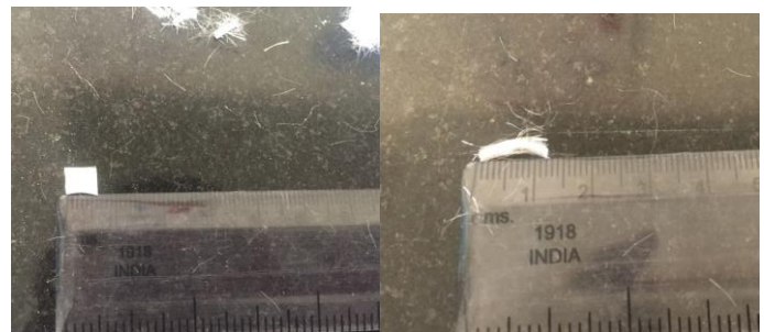
Figure.3. Polypropylene Fibres of 6 mm and 12 mm lengths
