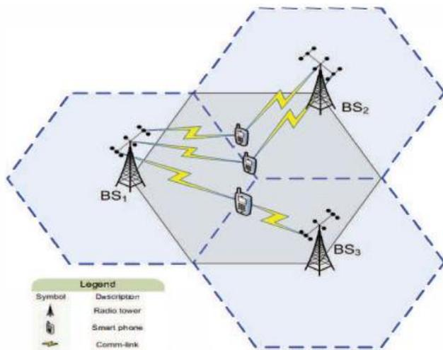
**Figure.2, Static cluster of three cells with Joint Transmission**
