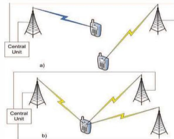
**Figure.1. (a) Co-ordinated Scheduling or Co-ordinated Beam forming (b) Joint Processing / Transmission.**
