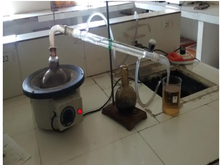
Figure.2. Schematic layout of Fractional Distillation Setup
