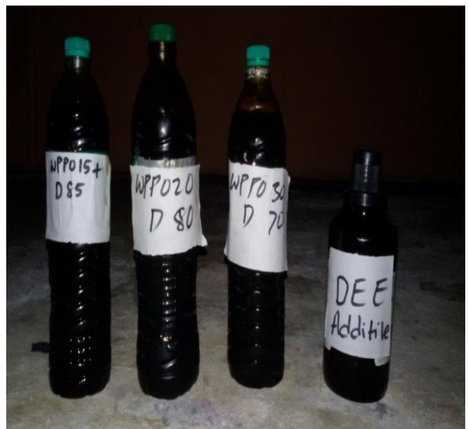
Figure.3. Tested samples of plastic oil with Diesel blends
