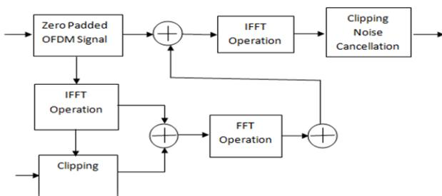
Figure.1. Block Diagram of Clipping and Filtering using noise cancellation
