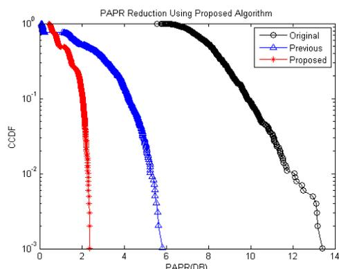
**Figure 5. CCDF of the PAPR for Clipping and Filtering with SLM**
