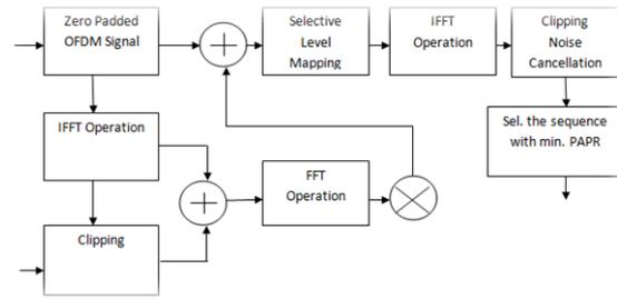
Figure.2. Block diagram of a Hybrid approach using CF and SLM technique with cancellation of noise to reduce PAPR
