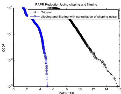
**Figure 4. CCDF of the PAPR for the clipping and filtering method with cancellation of noise**
