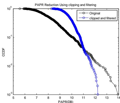
**Figure 3. CCDF of the PAPR for the clipping and filtering method**
