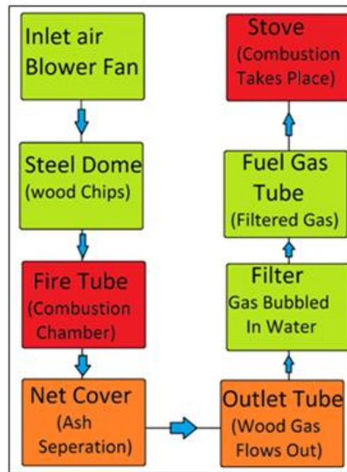
Figure .3. Block Diagram of the Wood Gas Gasifier
