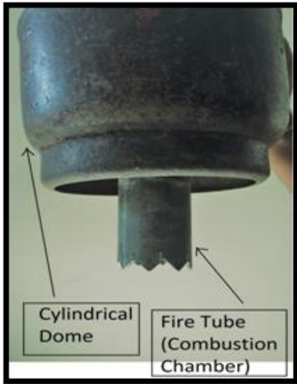
Figure 2.Cylindrical Dome and Fire Tube Of the Gaifier
