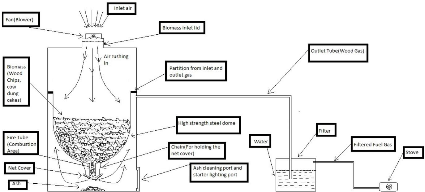
Figure.1. Working of the Wood Gas Gasifier
