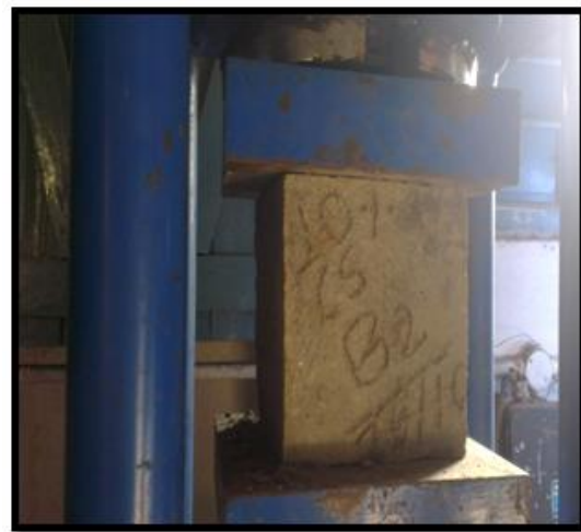
Figure .1.Testing of compressive strength of cubes
