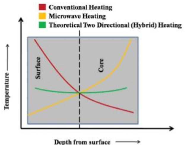
FIGURE 7.—Temperature versus distance profile for conventional, microwave, and two directional (hybrid) heating systems.
