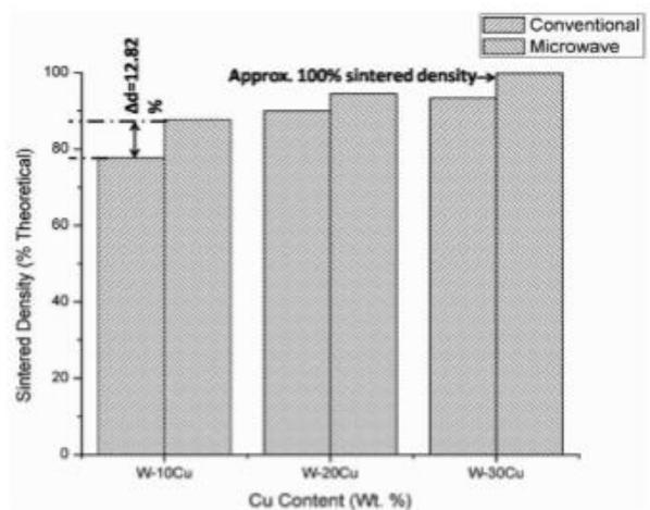
FIGURE 11.—Comparison of theoretical sintered density (%) of W–Cu composites under microwave and conventional sintering [50].
