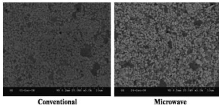
FIGURE 12.—SEM micrographs of W–Cu composite sample subjected to conventional and microwave heating [50].
