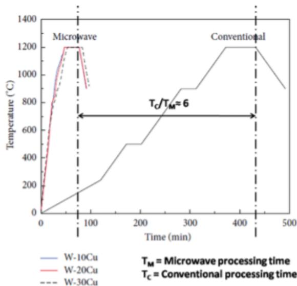
FIGURE 8.—Temperature versus time profile of W–Cu composites for microwave and conventional heating [50].
