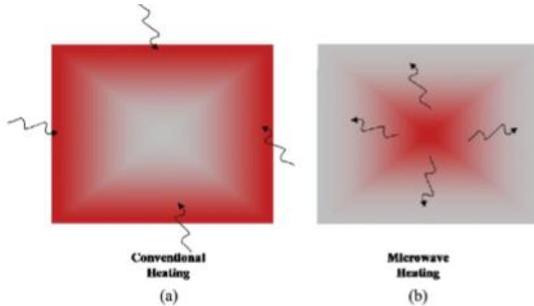
FIGURE 2.—Phenomenon of heat generation in (a) conventional heating and (b) microwave heating.
