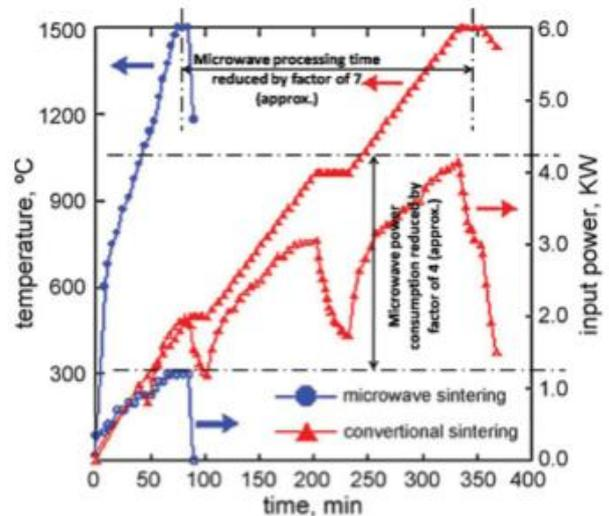
FIGURE 10.—Comparison of power consumption and heating time for conventional and microwave sintering [45]. © [Elsevier]. Reproduced by permission of Elsevier. Permission to reuse must be obtained from the rightsholder.
