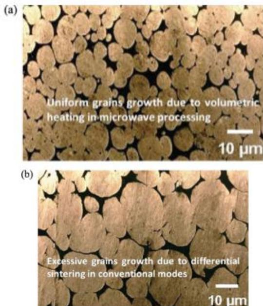
FIGURE 13.—SEM micrographs of (a) microwave and (b) conventional sintered tungsten alloy [45]. © [Elsevier]. Reproduced by permission of Elsevier. Permission to reuse must be obtained from the rightsholder.
