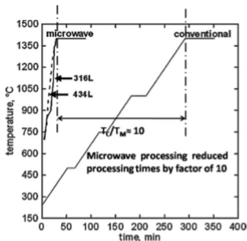
FIGURE 9.—Temperature versus time profile for 316L and 434L austenitic stainless steel under microwave heating and conventional heating [51]. © [Elsevier]. Reproduced by permission of Elsevier. Permission to reuse must be obtained from the rightsholder.
