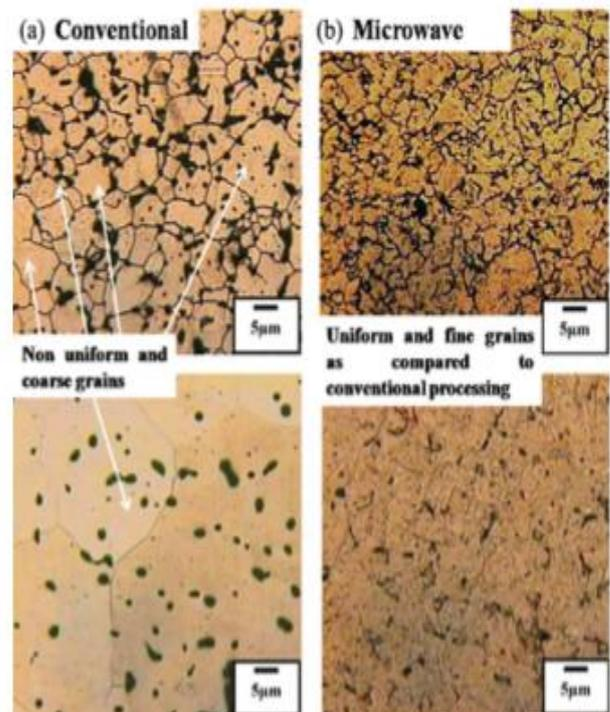
FIGURE 14.—Optical microstructure of 316L and 434L steel compacts sintered for 1 h at 1400°C in (a) conventional furnace and (b) microwave furnace [51]. © [Elsevier]. Reproduced by permission of Elsevier. Permission to reuse must be obtained from the rightsholder.
