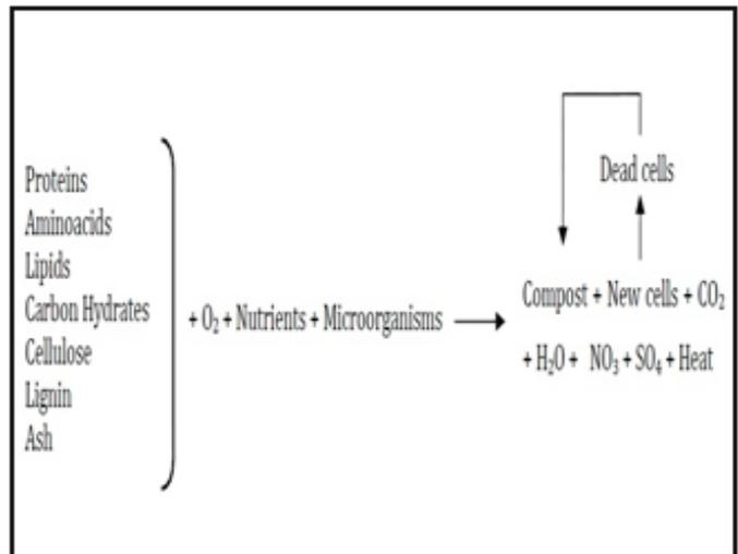
**Figure.4. Diagram of the composting process**
