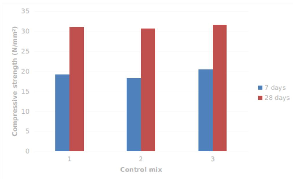
Figure.2. Compressive strength (N/mm<sup>2</sup>) of control mix
