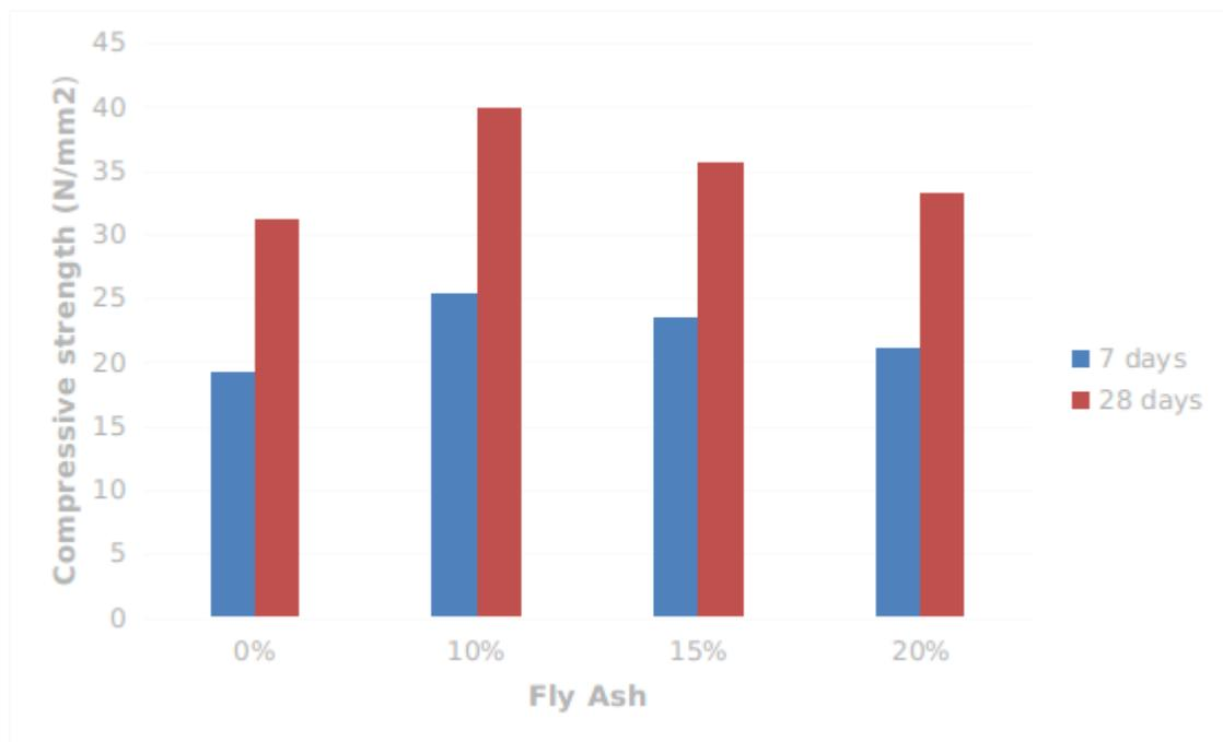
**Figure.3. Compressive strength (N/mm<sup>2</sup>) of different proportions of fly ash**
