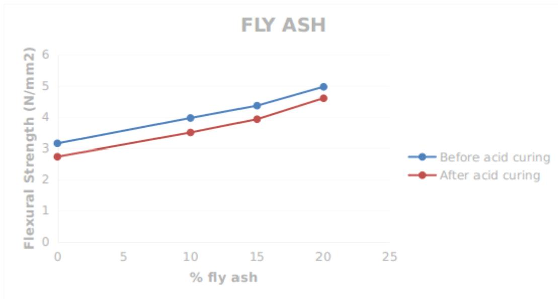
Figure.5. Flexural strength (N/mm<sup>2</sup>) of different proportions of fly ash
