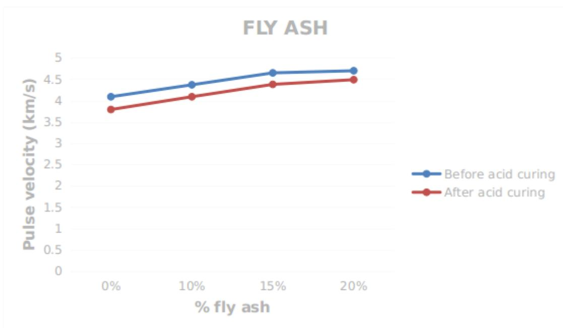
Figure.6. Pulse velocity of different proportions of fly ash
