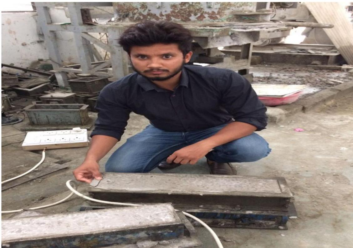
**Figure.4. casting specimen for Flexural Strength test**
