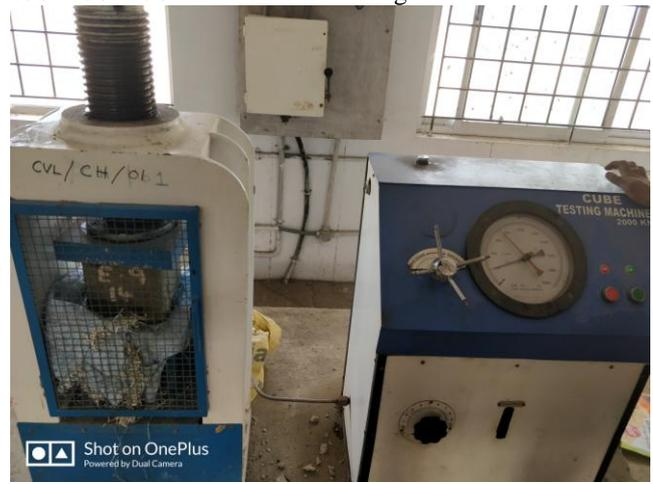
Figure.2. Compressive Strength Test.
