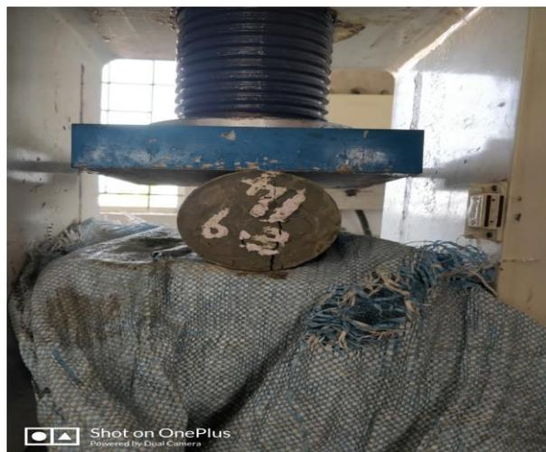
Figure.3. Split Tensile Strength.
