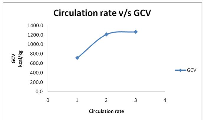
Figure 3.2.6 Effect of solid circulation rate on GCV.
