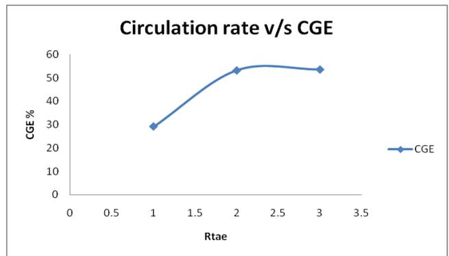
Figure 3.2.5 Effect of solid circulation rate on CGE
