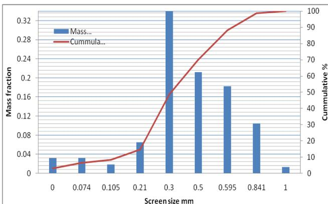
**Figure.2.1 Particle size distribution of bed material (Olivine) Mean particle size of bed material 0.3 mm**
