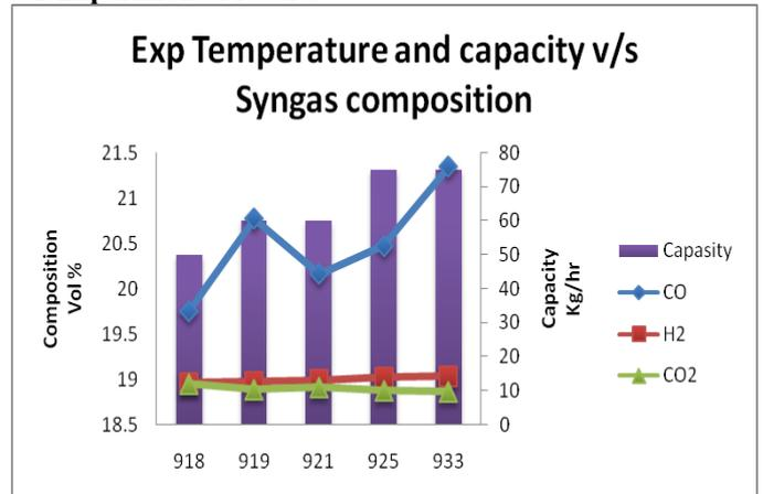
**Figure.3.1.1 Effect of gasifier temperature and coal capacity on syngas composition**
