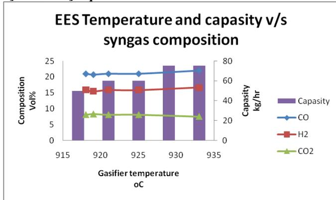
Figure 3.2.1 Effect of gasifier temperature and coal capacity on syngas composition
