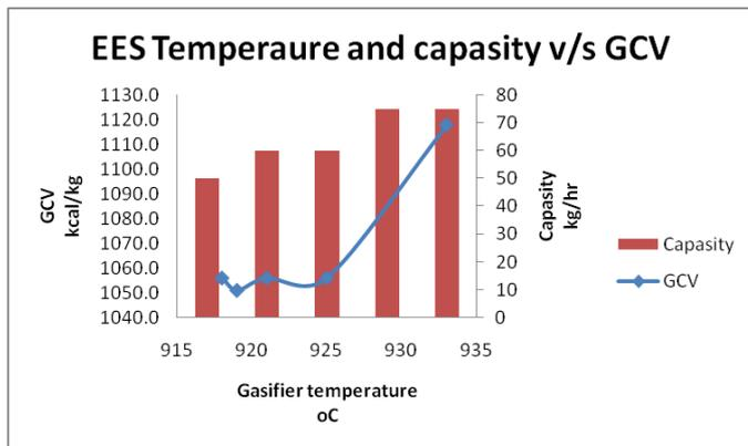
Figure 3.2.3 Effect of gasifier temperature and coal capacity on GCV.
