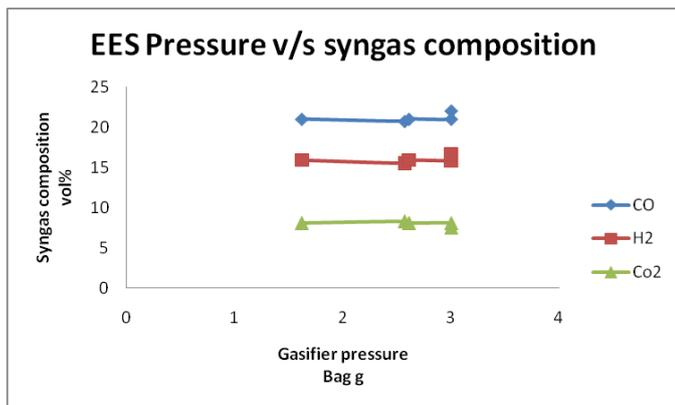
Figure 3.2.2 Effect of gasifier pressure on syngas composition
