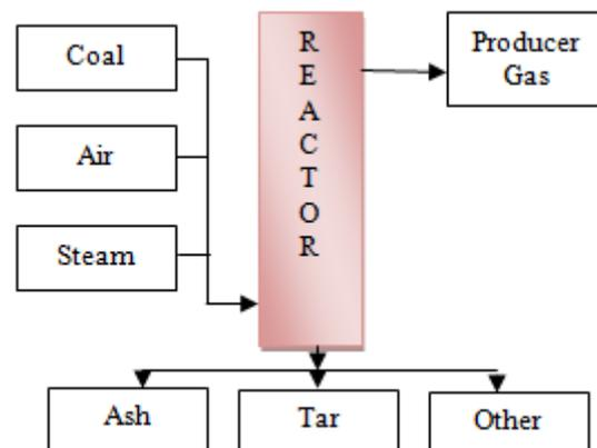
The overall material and mass balance taking around the gasifier as follow
