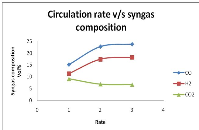
Figure 3.2.4 Effect of solid circulation rate on syngas composition
