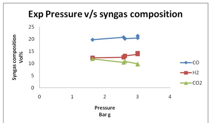
**Figure.3.1.2 Effect of gasifier pressure on syngas composition**
