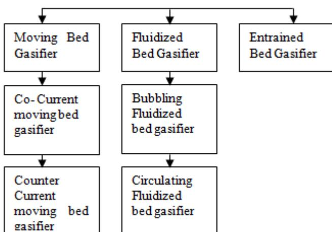
Figure 1.1 Types of gasifier reactor
