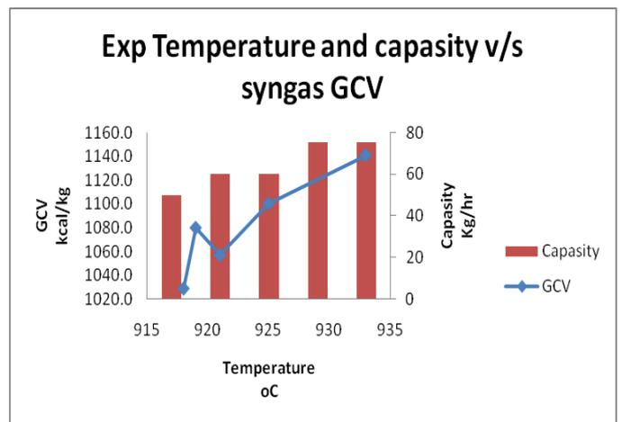
**Figure 3.1.3 Effect of gasifier temperature and coal capacity on GCV**
